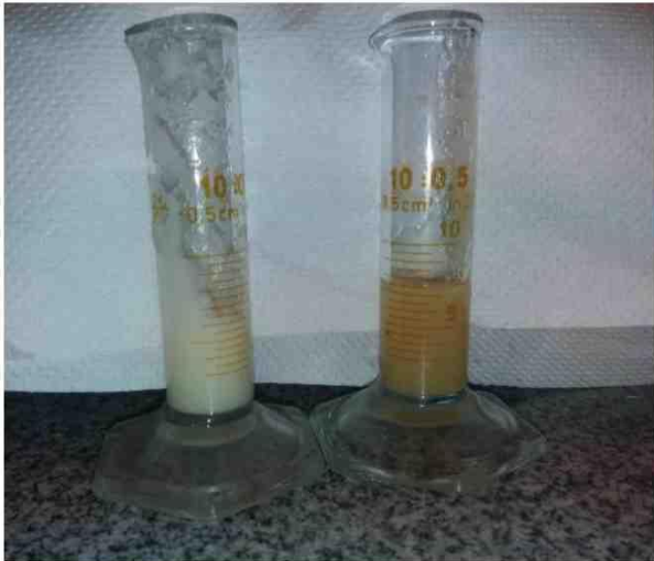
Figure 3. Aqueous garlic solution (40%) in measuring cylinders before heating (left) and after 30 minutes heating time (right).
